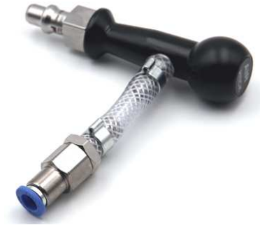
64-20630-29 1 pcs Compressed air plug (gas sampling plug) DIN 13260 with modification connection IQS standard (max. 10 bar) suitable for polyamide spiral hoses (blue or green)
