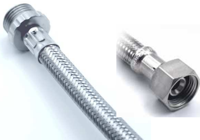
64-20815-20 1 pcs De-ionized waterhose / Drinking waterhose, length 100cm , AG1/2" and 3/8" connector for water supply 64-20815-21 1 pcs De-ionized waterhose / Drinking waterhose, length 150cm , AG1/2" and 3/8" connector for water supply 64-20815-22 1 pcs De-ionized waterhose / Drinking waterhose, length 200cm , AG1/2" and 3/8" connector for water supply 64-20815-24 1 pcs De-ionized waterhose / Drinking waterhose, length 300cm , AG1/2" and 3/8" connector for water supply 64-20815-26 1 pcs De-ionized waterhose / Drinking waterhose, length 400cm , AG1/2" and 3/8" connector for water supply
