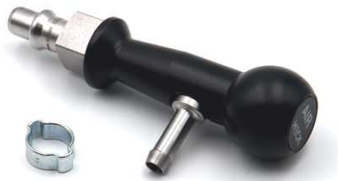
64-20630-25 1 pcs Compressed air plug (gas sampling plug) DIN 13260 with Jurid clamp suitable for PVC hoses
